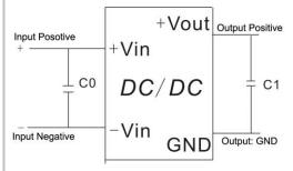
2. Input reflecting ripple current test circuit:
