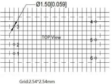
Grid:2.54\*2.54mm Unit:mm[inch] Pin tolerance: ±0.10[±0.004] General tolerance: ±0.50[±0.020]
