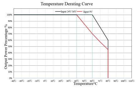
Note1: The temperature derating curve is based on the product with heatsink and no wind environment.
