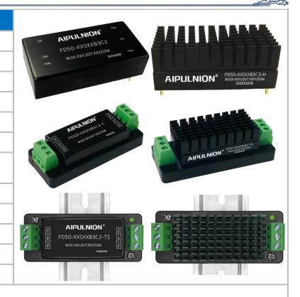
50W DC-DC Converter, 4:1 ultra-wide range input voltage, ultra-fast start, isolated stabilized voltage output, DIP/terminal post/rail packaging, single output. The isolation voltage is 1500VDC. It has the functions of input undervoltage protection, output overcurrent protection, output short-circuit protection, output overvoltage protection, etc., and is widely used in industrial control, electric equipment, communication, locomotive, industrial robot and other industries.
